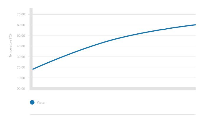
The graph above shows a test report on the HIBC/A heating 1000l of water.
