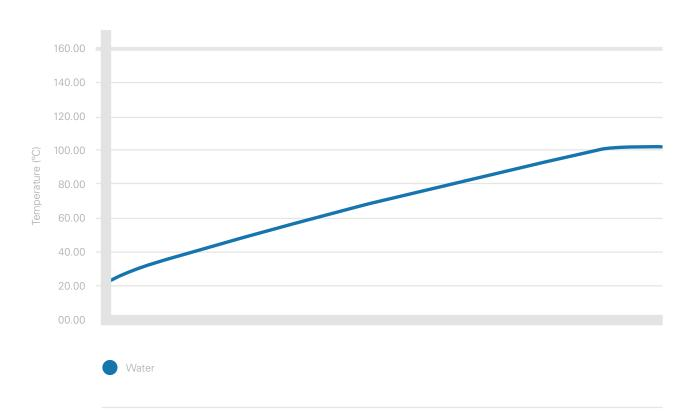
The graph above shows a test report of 3 x 1500W HSSD'S fitted to a 200l Steel drum.
