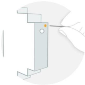
Press “Star Search” button and use a clip to press the small button placed at the top of the meter.
